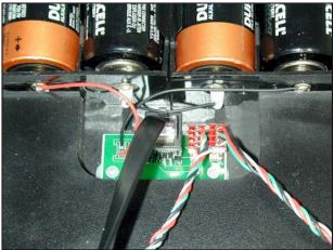
Control (left) and Motor (right) Connectors
