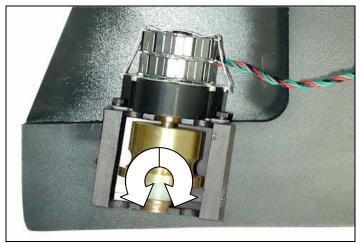
Rotate Brackets to Match Drive Wheels with Plate
