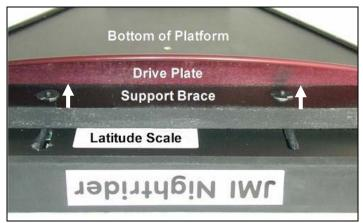
No Gap between Support Brace and Drive Plate
