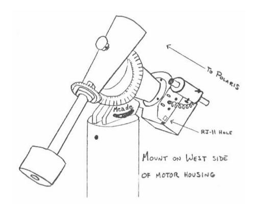
**EZAlign Installed on a Meade Equatorial Starfinder**
