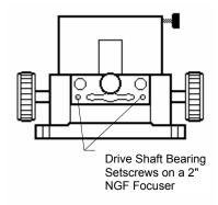
bearings, be made by the customer. Pusher bearing adjustments (between the drive shaft bearings on NGF-XTn, NGF-DX1 and NGF-DX2 models only) are extremely critical.
