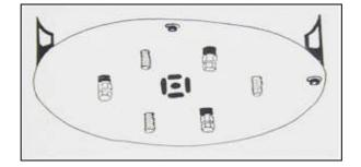
Bottom view of mirror cell, showing alignment studs
