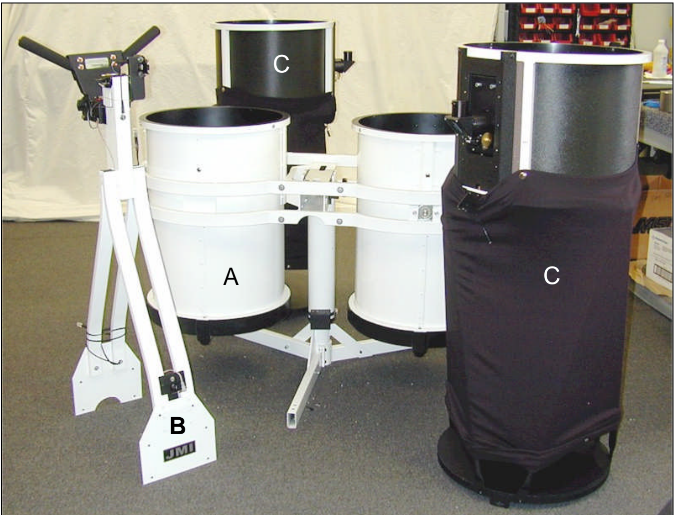
Figure 1 Tub and Pier section (A), Center Section (B) and Optical Tube Assemblies (C)
